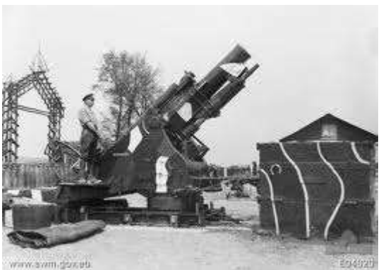
An unidentified British soldier standing with a 9.2 inch howitzer Mk I, named Berdamedia, which was supporting the Australians on the Somme. The camouflaged box in front of the gun is known as a dirt box, which was filled with soil and attached to the gun to act as a counterweight to the force of the blast and keep the gun in position. Hanging on the side of the box is a horseshoe. Note in the background (left) a timber structure, probably an observation tower and rows of shells in front of the structure.
